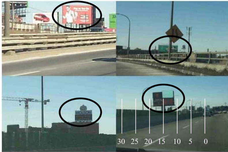
Figure 1: Photographs showing clockwise from top left: a Billboard sign, a Roller Bar sign, a Video Sign (sign # 67), and a Scrolling Text sign (sign # 64). The bottom right picture shows the 5-degree increments used to measure the glance angle. The sign, as depicted, is at 15 degrees (NB: increments may not be to scale).
